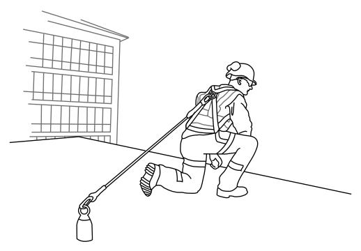
Figure 1 — Fall restraint
